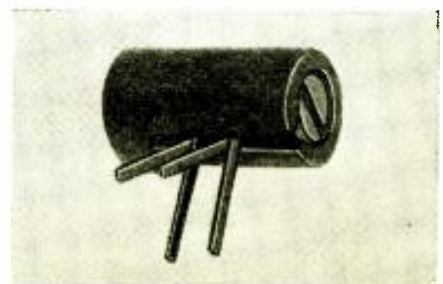
A metal-oxide rectifier. A metallic film provides contact to the oxide. (No. 409)
